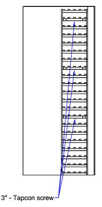
For uneven surfaces, like brick, we recommend using a slotted "L" bracket that you secure to the post with a 5/8" screw and then use a Tapcon screw to secure to the wall.
